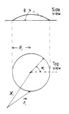
**Figure 1.** Geometry of the *i*th cap-shaped nucleus growing on a substrate.
